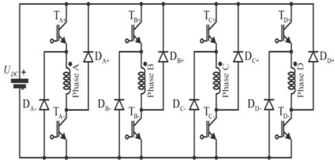
Fig 1. Asymmetric converter for four phase SRM.
