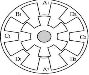
Fig 2. The SRM 8/6 Construction
